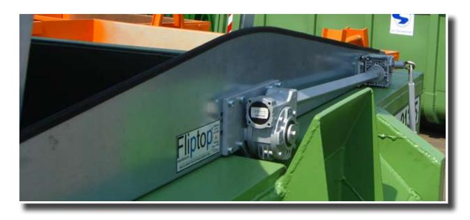
Fliptop - Gear opens from one side and folds together on the opposite side.
